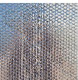
Our most popular insulation solution consists of a high performance industrial bubble layer with entrapped air, on its outer surfaces are two highly reflective layers of aluminium coated with an ultra thin protective surface to protect the aluminium for the life of the product. This product is around 4mm thick and is equivalent to around 55mm of Polystyrene
