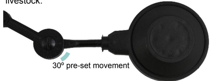
This is the pre-set articulation point that allows the tank level to decrease, without opening the regulator. This works because the arm allows the float to move before the arm engages with the regulator.
