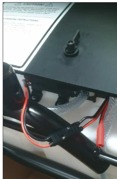
Connection if using the built in battery
