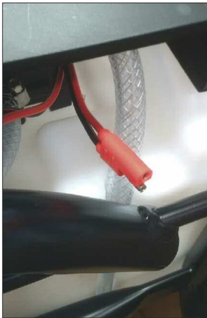
Connection if using from external power source for the pump e.g. ride on lawn mower
