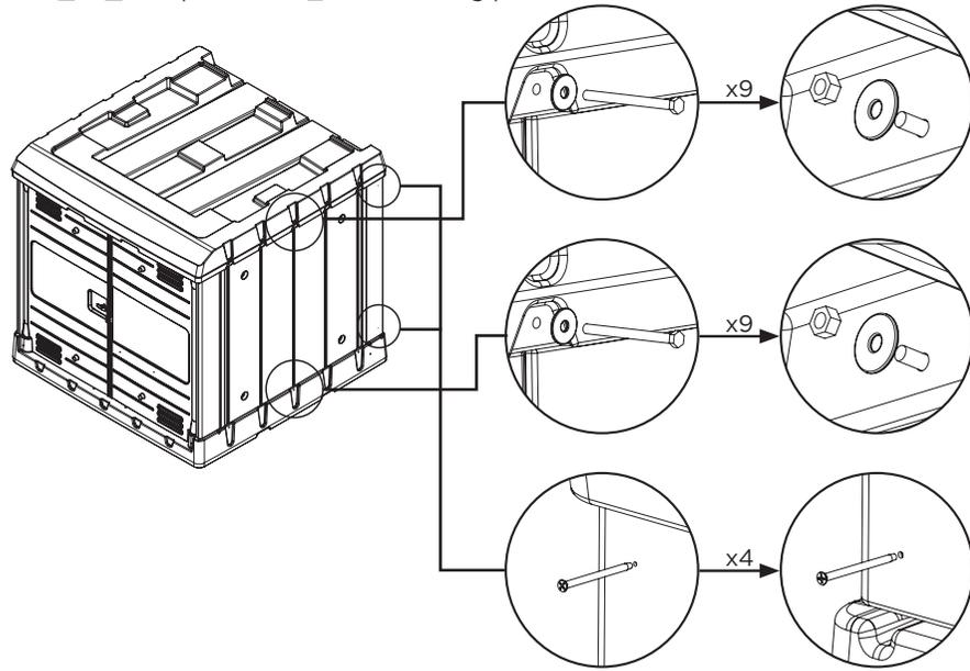
8. **IMPORTANT!** Make sure spill pallet central supports are in place before completing assembly
