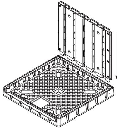
3. Insert **C** into **A** (one at a time) making sure corner joints intersect
