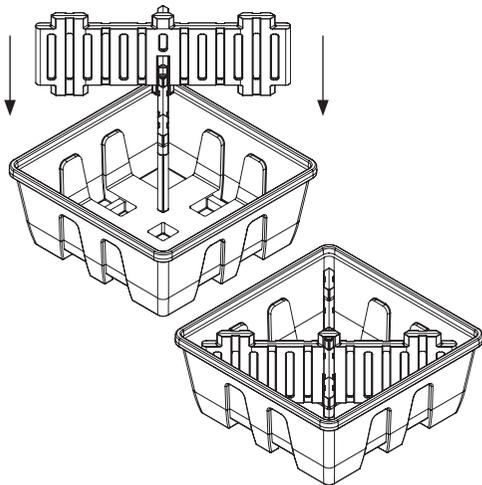
9. Forklift IBC Hardcover onto spill pallet central supports using forklift pockets, making sure platform aligns with central supports
