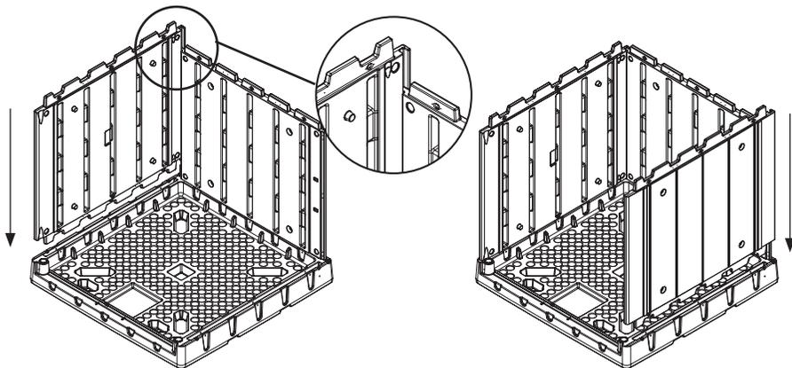
4. Forklift **D** onto **B** & **C** making sure **B** & **C** locate into **D**
