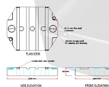
The Oaklands Rhino effluent tank has been designed to meet the needs of the portable sanitation industry. Its low profile design allows it to be positioned alongside or underneath portable site accommodation, toilet blocks, kitchens, canteens and welfare units.
