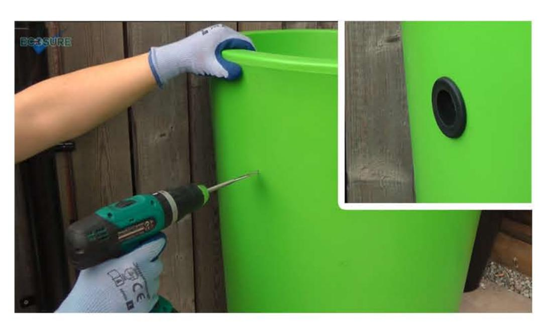
b. Using a 26mm hole-saw or spade bit, cut a hole just below the base of the planter bowl and insert the rubber seal.
