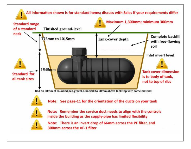
NB: Before commencing the dig, ensure invert-level + 300mm is not less than 500mm or more than 1300mm if the tank is to be unprotected.
